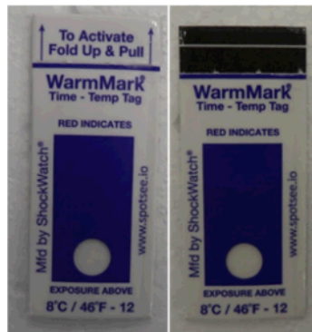
Figure 12c Inactivated vs. Activated temperature indicator.
