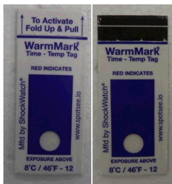
Figure 12c Inactivated vs. Activated temperature indicator
