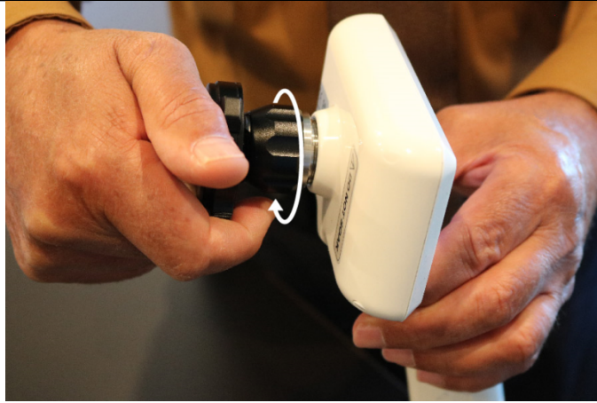
Figure 17 Aligning the endobody clamp with the camera
