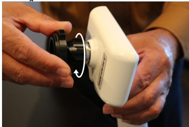
Figure 16 Connecting the coupler and camera head
