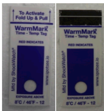
Figure 12c Inactivated vs. Activated temperature indicator
