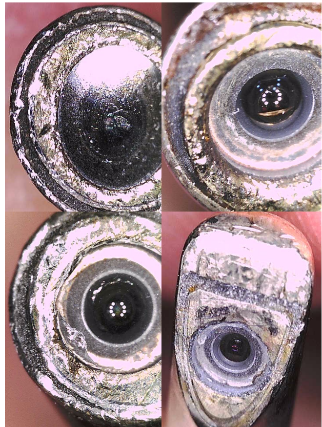
Figure 6: Identified with the use of an enhanced magnification microscope (exposed burrs, gouges, recessed areas, and scratches)
