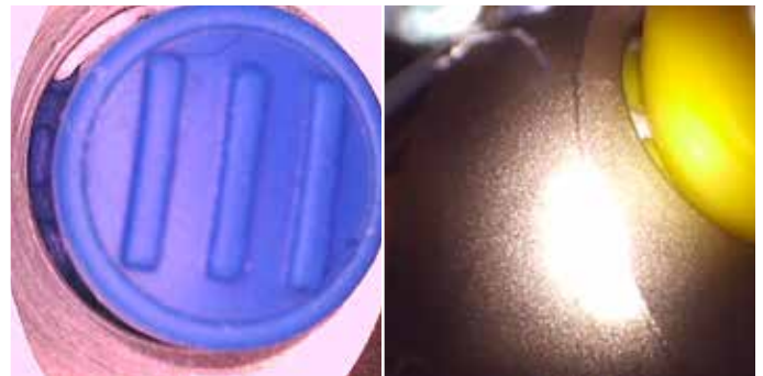
Figures 8A and B: Identified external debris (around the buttons) with the use of an enhanced microscope
