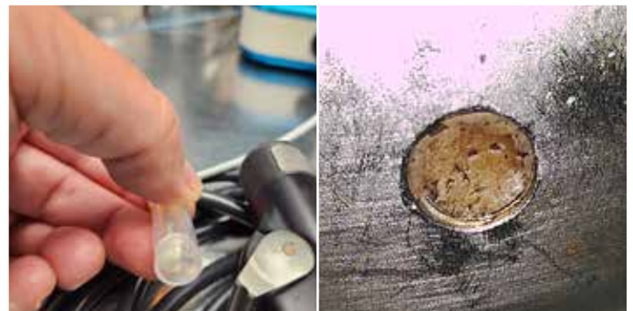
Figure 10A & B Identified external debris that tested positive for residual protein (damaged silicone insert)
