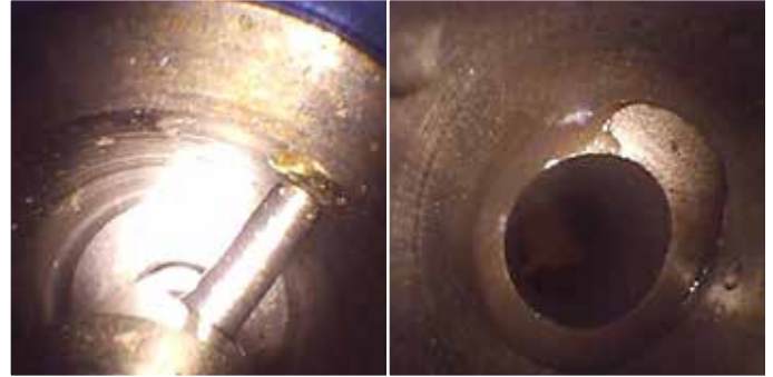
Figures 6A and B: Identified internal debris with the use of a borescope
