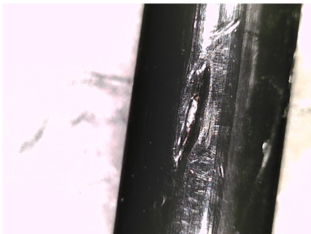
Figure 1: Integrity failure in an insulated laparoscopic shaft.
