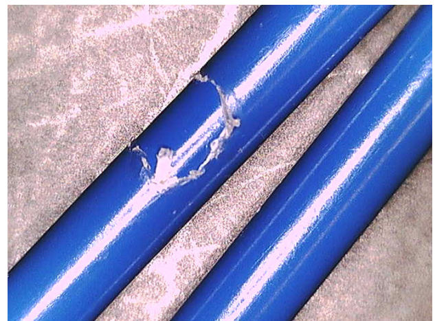
Figure 2: Insulated bipolar forceps failures.
